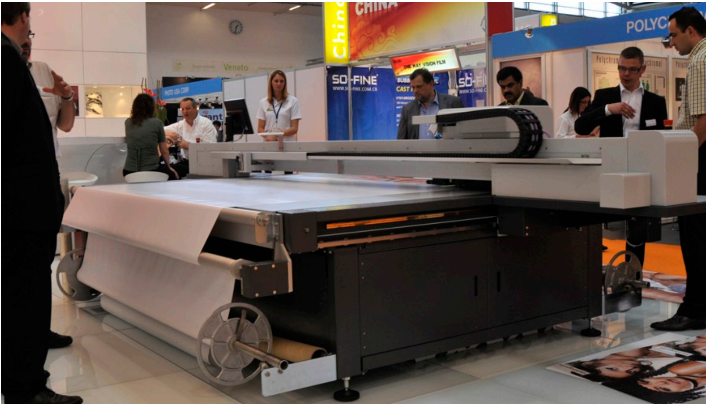
Rear view of the SwissQprint Impala UV flatbed printer at FESPA 2010. In this model roll media is loaded at the back.
